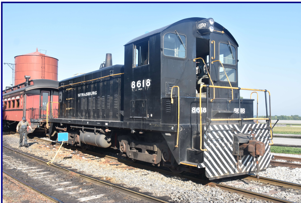
Strasburg Railroad SW-8 8618, nee New York Central 9618, built by Electro-Motive Division in 1954.
