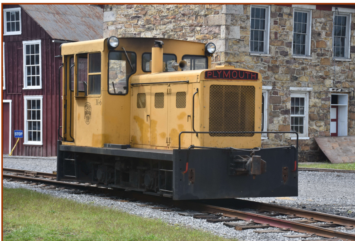
East Broad Top 12 ton switcher M-6 built by Plymouth in 1968.
