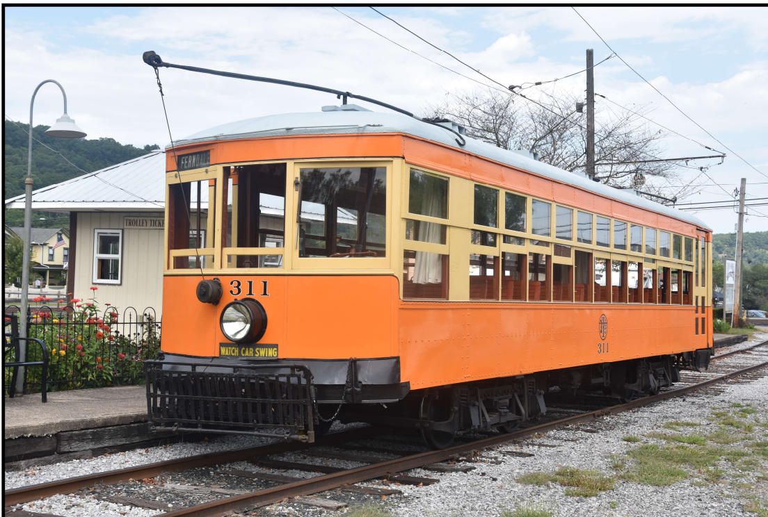
Johnstown Traction Company double-truck Birney "safety car" 311 built by Wason in 1922. It was part of an order of cars for the City of Bangor, Maine, where it operated as number 14. It was sold to the Johnstown Traction Company in 1941 and served that city well, running until the end of service in 1960. Car 311 was the last Birney type car to be operated in any United States city on a regular schedule and was chartered repeatedly by trolley fans in the 1950's, as it was a favorite car of many.
