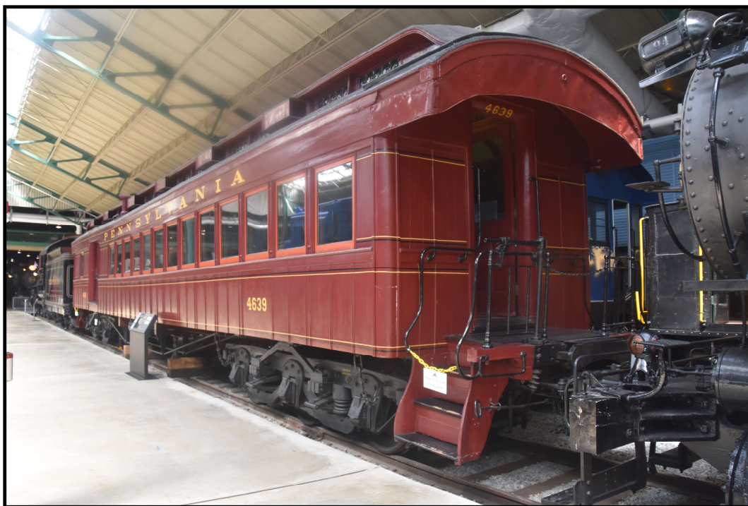
Pennsylvania Railroad baggage combine "4639" built by the railroad in 1894. Complete with ornate kerosene lamps and coal stove, this car was outshopped with six-wheel trucks for heavy-duty mainline service. This car has been displayed at world's fairs and transportation exhibits from coast to coast.
